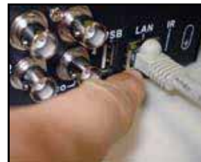
Figure 1.2 Connect the Ethernet cable
